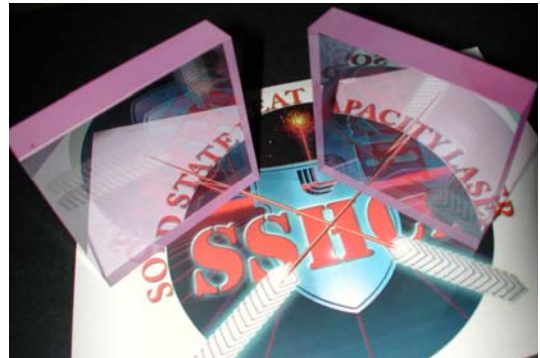
Fig. 2. Ceramic YAG slabs. The dimensions of the slabs are 10 \times 10 \times 2 cm 3 .
